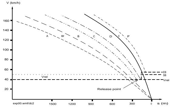
*Note*. The DE curve is drawn to zero. There is not, however, any supervision function below the release speed with the exception of providing a reference for the ABf and the BfB curves.
