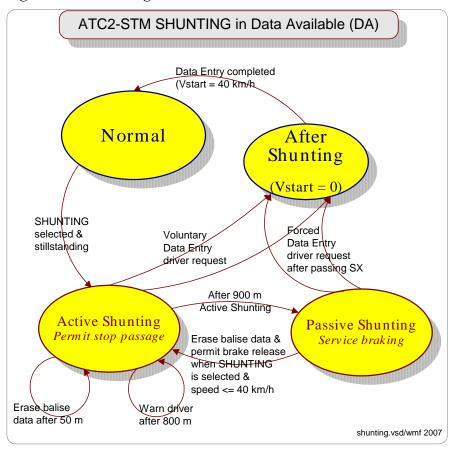
Figure 4.3-3. Shunting state machine
