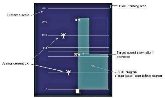
A-note. The Target Speed and Target Distance (TSTD) diagram.
