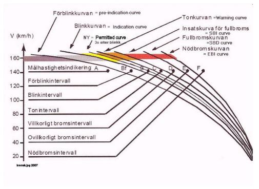
Figure 4.6-4. Braking curve intervals that affect the indications
