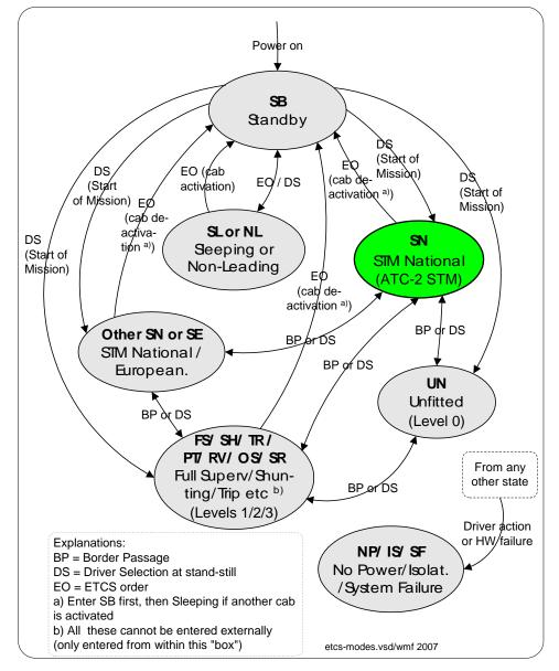
Figure 4.3-2. ETCS Mode & Level Transitions Overview
