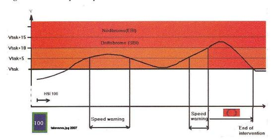
Figure 4.5-1. Max speed supervision with MARGIN BAR colours
