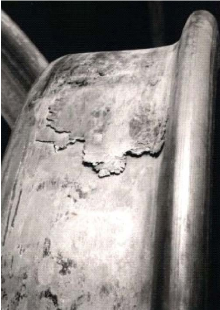
Metal build up on the tread
