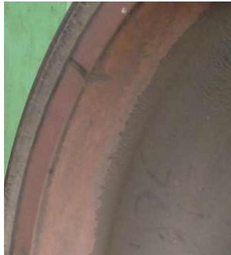
Old and fresh burnt paint
